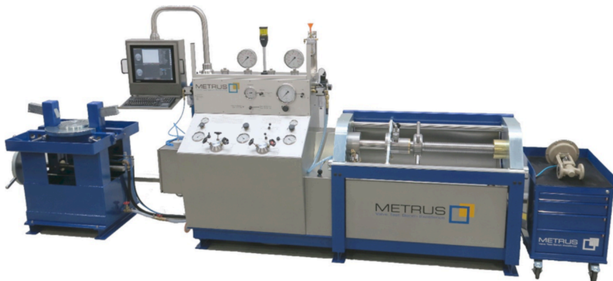
Figure 2: Combined test benches are versatile and can be used for a wide range of valves.
